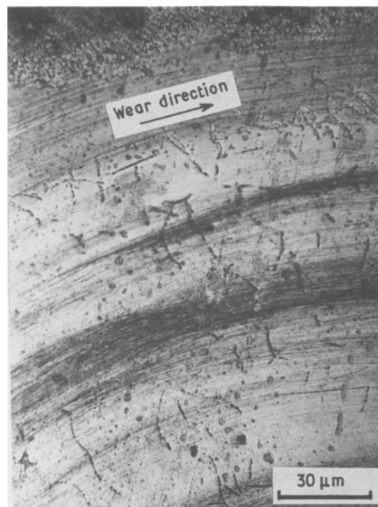
Figure 8 Optical micrograph of worn chromium deposits, d.c. plated at the current density of 1 \text{ A cm}^{-2} .
